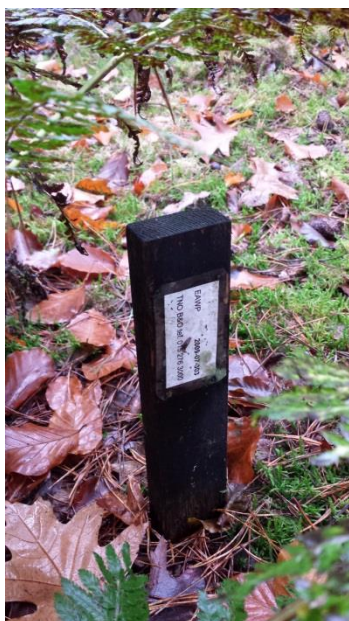
Figure 2: In ground test according to EN 252
