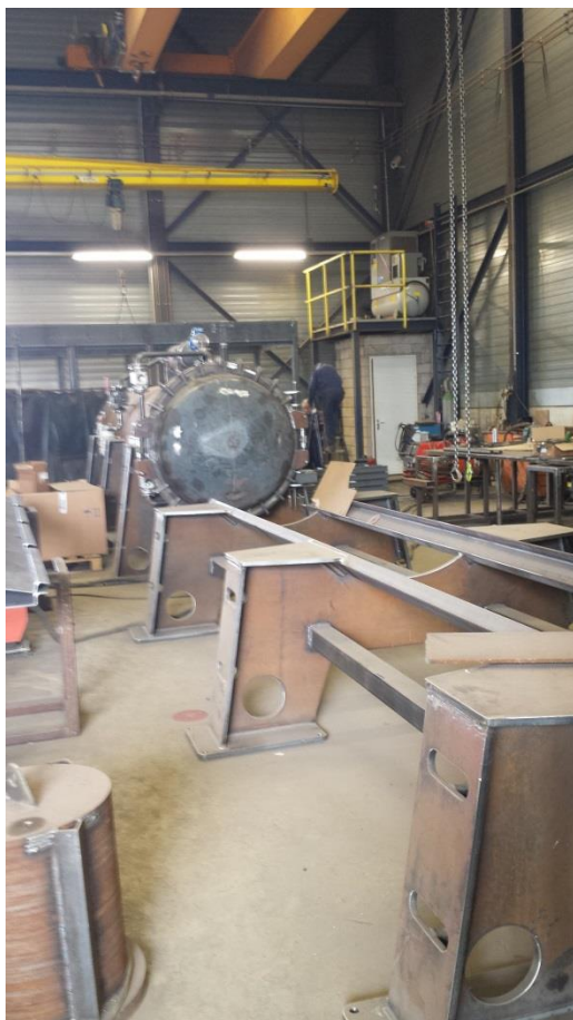
Figure 8: Construction of the 4m 3 pilot impregnation plant at van der Zalm B.V. Foreground: the rails for loading the vessel
