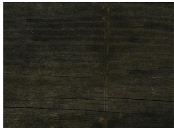
**Fig. 2.** The wood piece is covered with a uniformly coloured biofilm.
