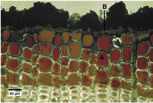
Fig. 3. Biofilm on treated wood after 36 months exposure (magnification 100×).
