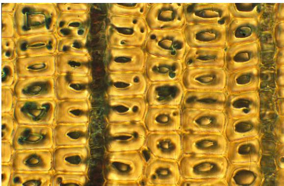
Fig. 4. Degradation pattern of untreated pine sapwood reference after 36 months exposure (magnification 100×).
